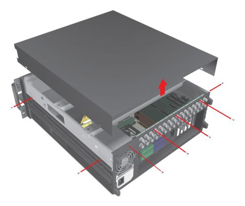
Figure 4. Removing Chassis Cover
